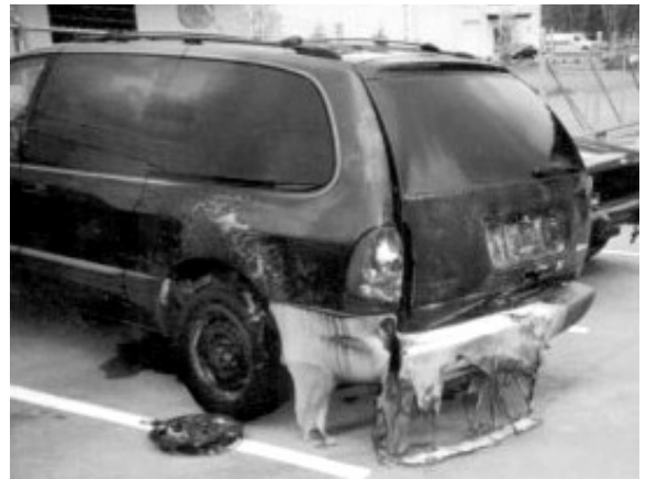
Damage done to a vehicle from a fire started by static electricity.
